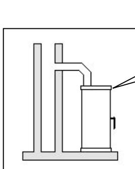
The fireplace can usually be connected to the chimney with an angle pipe
